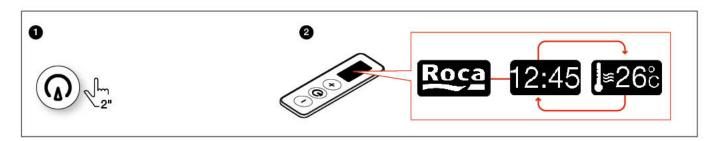
If there is not any active functions reverts to Stand by mode, after a minute or press this key (a) during two seconds.
