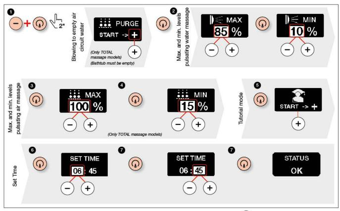
It returns to main screen if you do not press any key during ten seconds or press the key ((a)) during two seconds.
