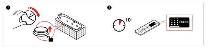
After 10 minutes emptying the bathtub after using the whirlpool, it automatically activates the blowing process, if not previously done manually blowing.
