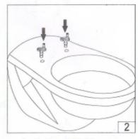
Insert the hinge set into the hole.
