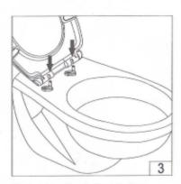
Keep the toilet seat in vertical, insert the hinge, adjust the seat cover to suit the toilet, make it in suitable position then pull off the seat cover in vertical.
